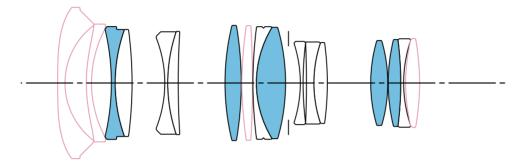
17 Elements in 12 Groups SLD (Special Low Dispersion) Glass :Aspherical Lens
